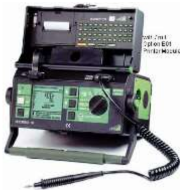
Picture: example for electric safety tester based on IEC601-1.
