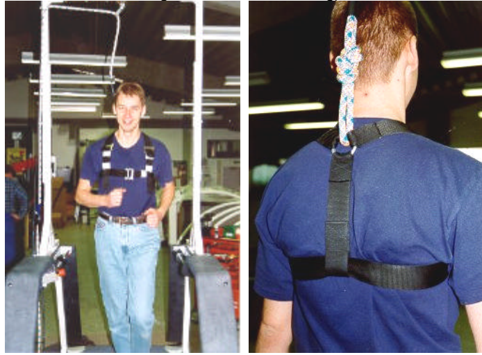
Illustration 7: Safety Arch with Harness and Chest-Belt-System
