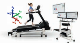
gait analysis / biomechanics gaitway® 3d with force and pressure measurement
