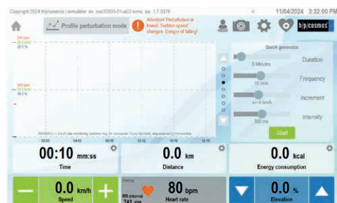
quick generator for quick and reliable adjustment of perturbation parameters
