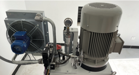
Hydraulic motor and oil tank for elevation adjustment
