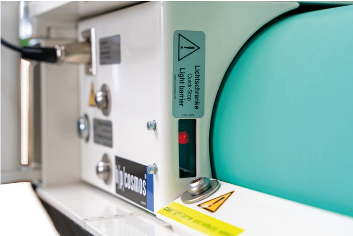
Light barrier for automatic emergency stop
