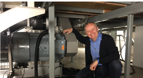
30kw drive motor for the 402kg heavy running belt below "the beast" - in comparison Mr. Franz Harrer
