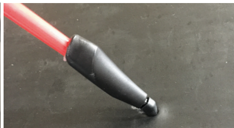
Surface of the treadmill belt gives way when using it with a ski pole
