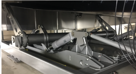
Hydraulic cylinder construction for dynamic and programmable elevation adjustment in different speeds
