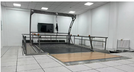
Properly fitted saturn® 450/300rs including stage floor and electric access ramp with wooden cover
