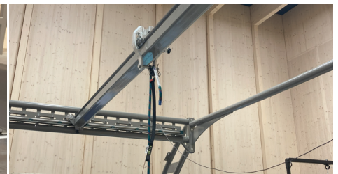
Safety harness system for free movement on the entire-treadmill belt length
