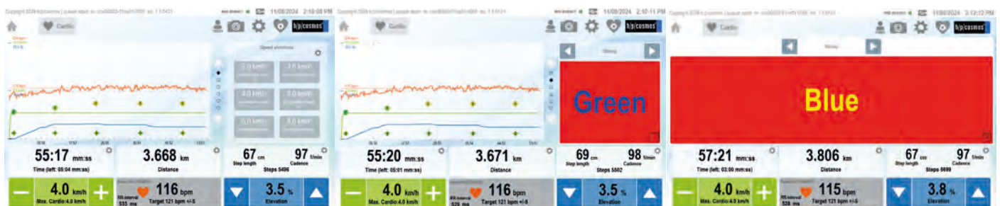
Multi-purpose display allows a wide range of additional information and tests, e.g. programmable speed shortcuts, or optional dual tasking and cognitive tasks. The display for optional dual tasking screens or cognitive tasks can be extended to the full screen while keeping all important training parameters in scope.
