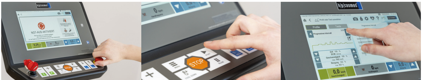
The combination of a 10.1" TouchScreen and a hardware keyboard allow an anytime secure handling of the treadmill - especially in situations of urgency.
