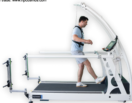
The perturbation mode called „shake“ will allow sudden speed changes to simulate slips and trips on h/p/cosmos MCU6 treadmills.
