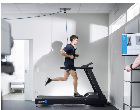
Instrumented h/p/cosmos treadmill with ceiling-mounted fall prevention
