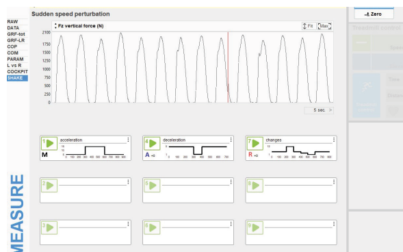
The perturbation mode called „shake“ will allow sudden speed changes to simulate slips and trips on h/p/cosmos MCU6 treadmills.
