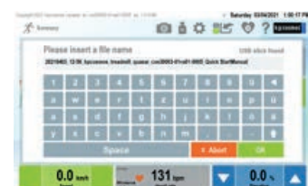
Summary report can be saved in PDF and .csv format with automatically generated informative and editable file name to the connected USB stick.
