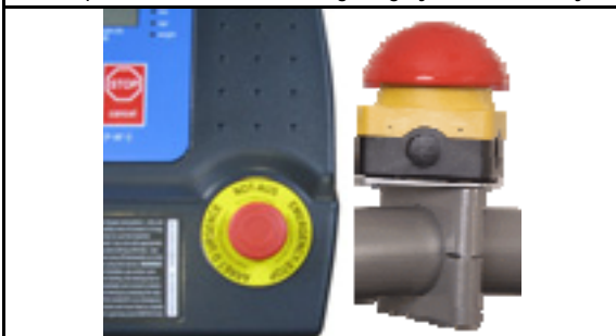
Emergency stop button on the UserTerminal. Triggers bi-polar disconnection from the mains (power supply). Additional emergency stop push button can be mounted on the opposite handrail of the treadmill.
