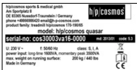
name plate of a sports device with 1-phase power supply example: h/p/cosmos quasar®
