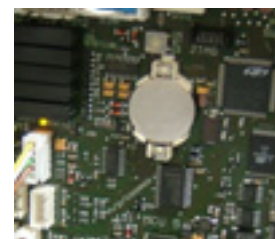
Picture: battery [cos12542] on the MCU5 circuit board
