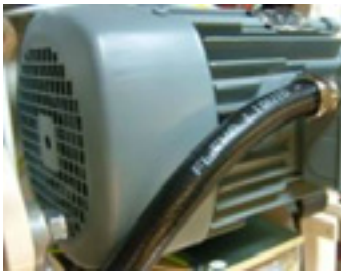
Shielded motor cable
