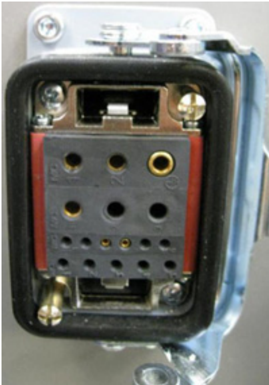
cos100710 socket in UserTerminal for inverter, drive and elevation motor
